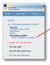
In the VPR system integrated cold storage controllers will be displayed in the VPR directory under "Cold storage controllers".
